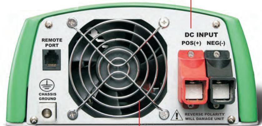
**Ventilation port:** Loading Controlled Cooling Fan (turns on at 149°F (65°C) and turns off at 113°F (45°C))
